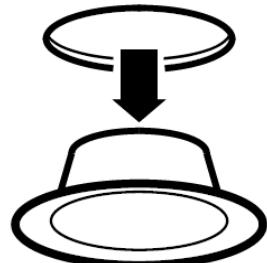
Isolate power supply then remove existing downlight
