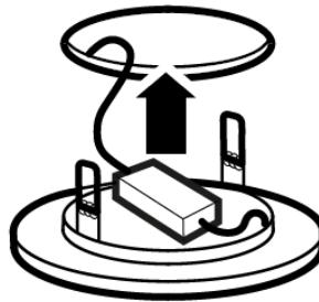
Place driver on panel, fold up spring clips and insert
