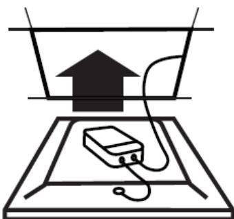
Place driver on to the panel then insert the panel back into the ceiling.
