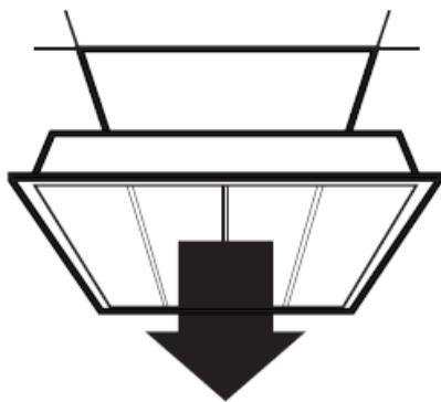
Isolate power supply then remove existing luminaire or ceiling tile.
