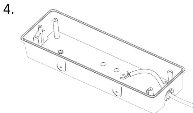
Feed the mains cable through the chosen entry point. Options for cable entry include rear central BESA cable entry (requires drilling) or end cable entry (use IP65 grommet).
