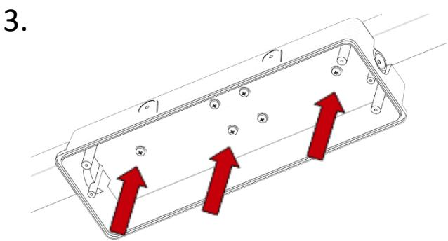
Attach the housing to the designated trunking or ceiling using chosen method. BESA fixings can be drilled and used or a simple two-point fixing can be utilised.
