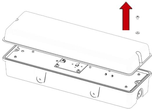
2. Remove the four screws from the gear tray and lift from the body.
