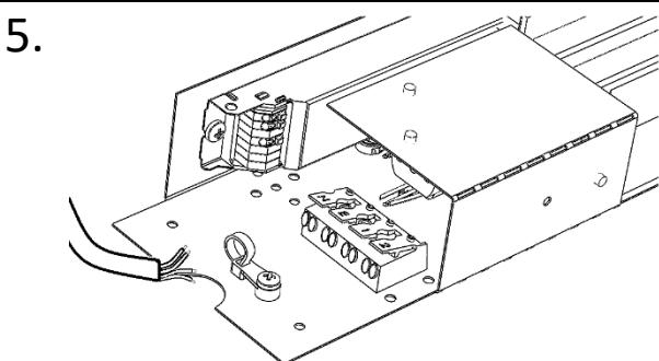
Wire the mains cable into the respective terminals on the terminal blocks provided taking care that the correct wires are connected to the correct terminals.
